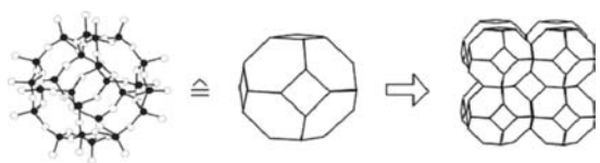
Figure 1: Schematic view of the sodalite structure, the basic cage and the connection pattern. Full and open circles refer to Al, Si and oxygen, respectively.
