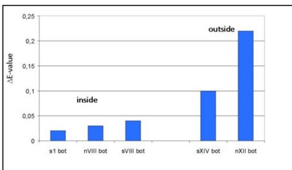
Figure 9: Glass sensor study in León (Spain): sensor positions (different windows, only bottom position) and corresponding stress levels detected on glass sensors ( $\Delta E$ -values) for unprotected windows
