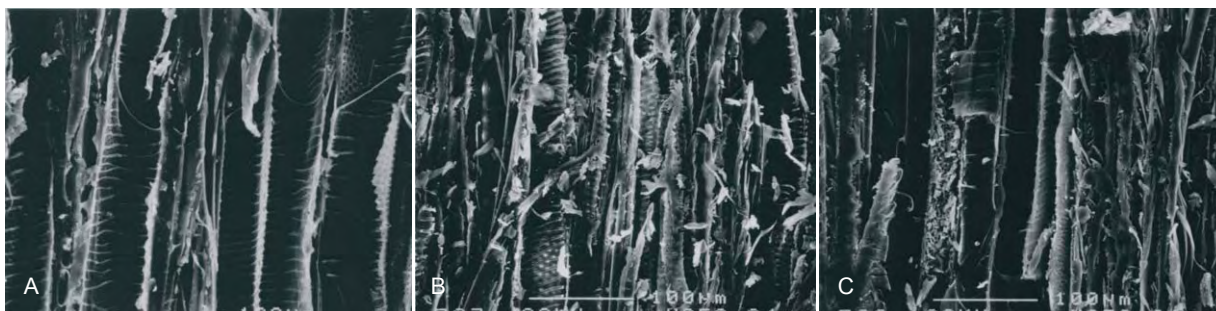
Figure 4. SEM micrographs of lime wood samples at a magnification of x250.
