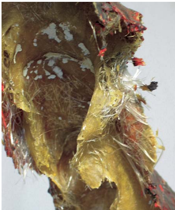
Figure 6: The yellowed UP composite layers from the dogs of the installation by Tykkylainen (Fig. 2).
