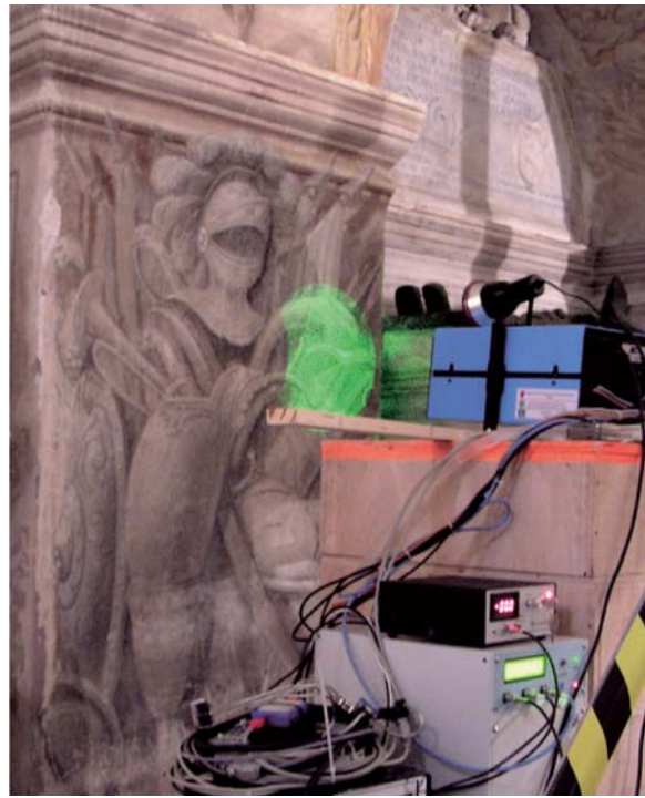
Figure 5: Left: transportable digital speckle holographic interferometric (DSHI) system (Benaki Museum, Athens, conservation lab), right: pulsed DSHI for in-situ applications (St Johns co-Cathedral, Malta).
