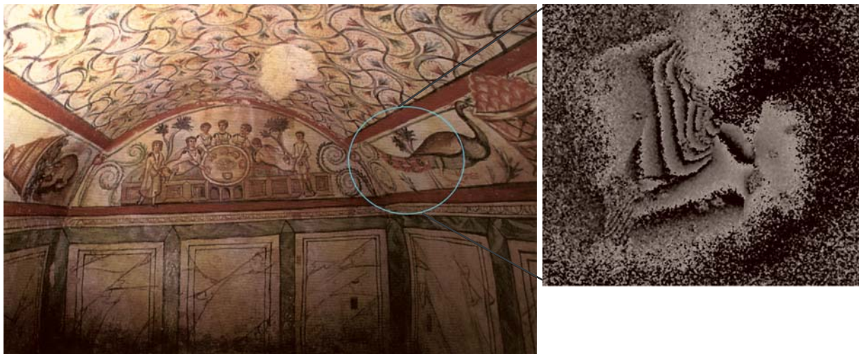
Figure 6: A study of defect detection in wall paintings in a crypt in Constanza, Romania. Right: an example of the detected detachment.
