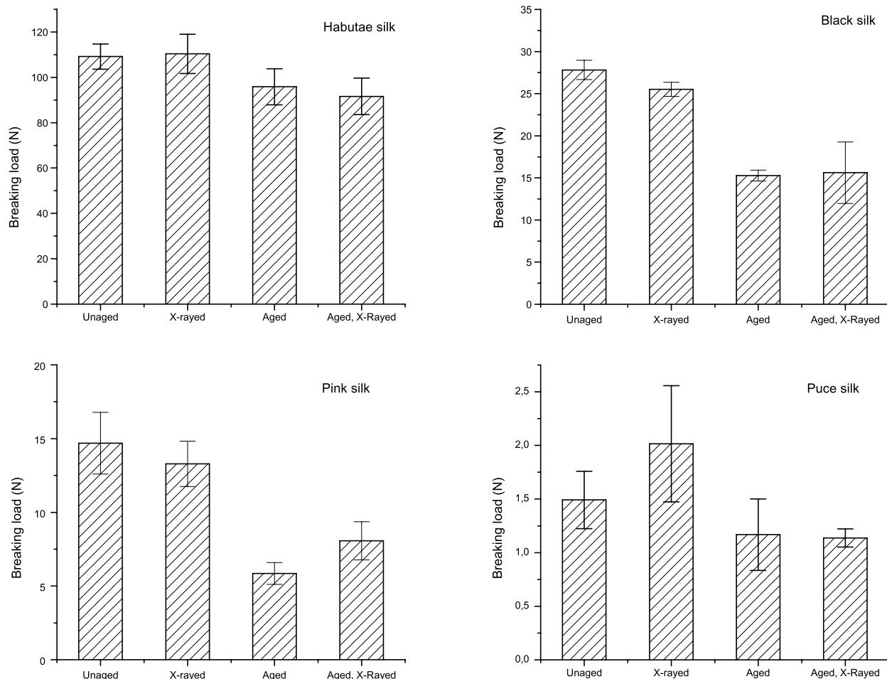
Figure 4: Average breaking loads of silk samples, with error bars based on the range of results.
