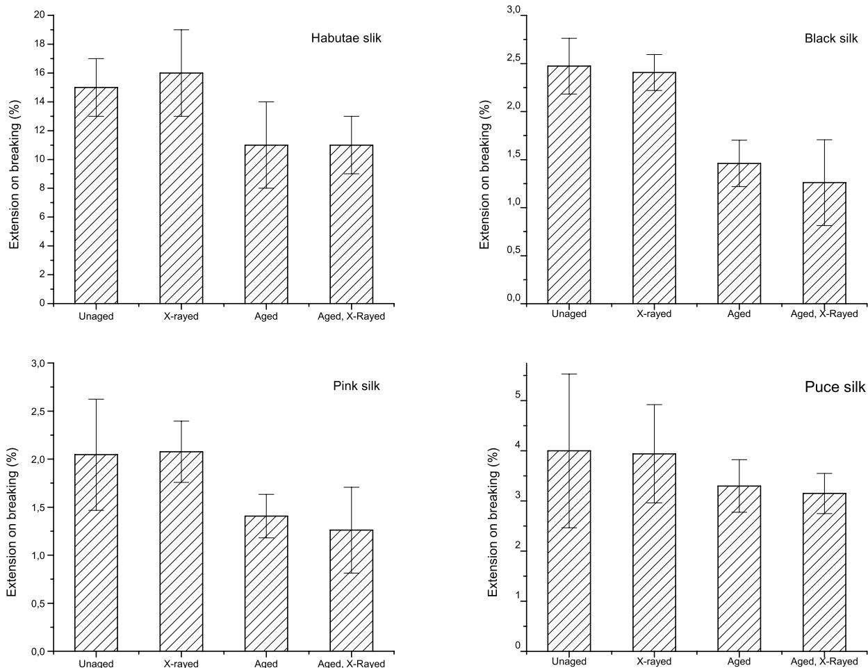
Figure 5: Average extension on breaking for silk samples, with error bars based on the range of results.
