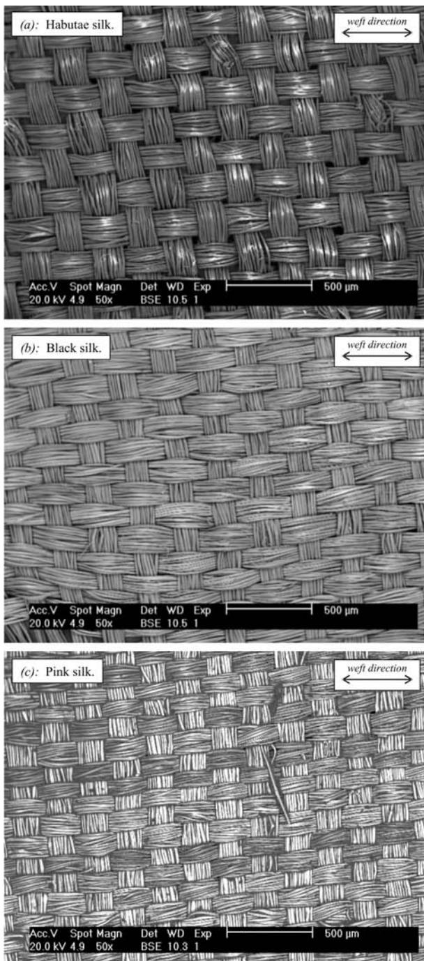
Figure 3: Back-scattered electron images of silk samples, showing representative samples of (a) an unweighted fabric, (b) a fabric in which the warp and weft yarns are uniformly weighted, and (c) a fabric in which the warp and weft yarns are weighted to different degrees.
