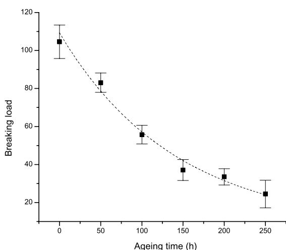
Figure 6: Average breaking loads of light aged habutae silk samples, with error bars.
