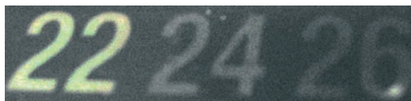
Figure 13: A photograph of a liquid crystal thermometer immediately after being irradiated with the microfademeter. Note 22 is clearly visible at 22 °C room temperature and the bottom right hand corner of the 26 showing a small circular area which has been increased in temperature to approximately 26 °C by the focused probe.
