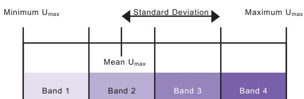
Figure 3: Arbitrary method used to divide the total range of moisture content values for each species into four "bands".
