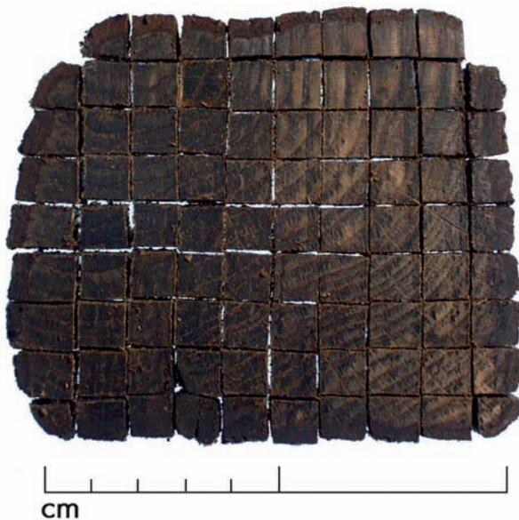
Figure 2: Timber section after cutting to produce individual 1 cm cubes.
