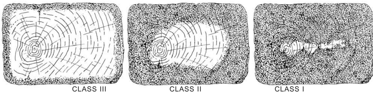
Figure 1: De Jong's classification for the degree of degradation of European oak. Adapted from ref. 18. CLASS III - "Wood containing <185% water". Sound core beneath a thin deteriorated layer. CLASS II - "Wood containing 185 - 400% water". Comparatively small core present. CLASS I - "Wood containing >400% water". Highly degraded wood predominates.
