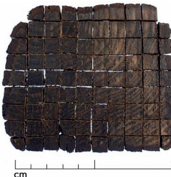
Figure 2: Timber section after cutting to produce individual 1 cm cubes.
