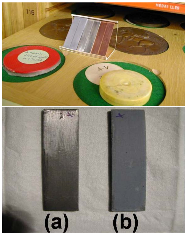
Figure 1: Setup for the exposure; on the top - coupons exposed at the Bibliothèque Nationale, cabinet des médailles, Paris; on the bottom- lead before (a) and after exposure (b).
