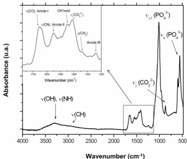
Figure 2: ATR-FTIR spectrum of a modern bone material (MBB) with bands assignments.
