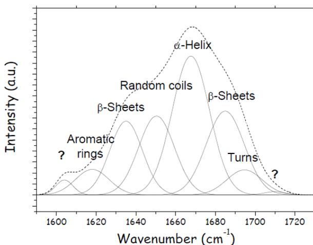
Figure 5: Curve-fitting analysis of the amide I profile of MBB in FT-Raman. Identification of the eight components (aromatic rings, two times  $\beta$ -sheets, random coils and  $\alpha$ -helix, turns and two non-attributable minor components).
