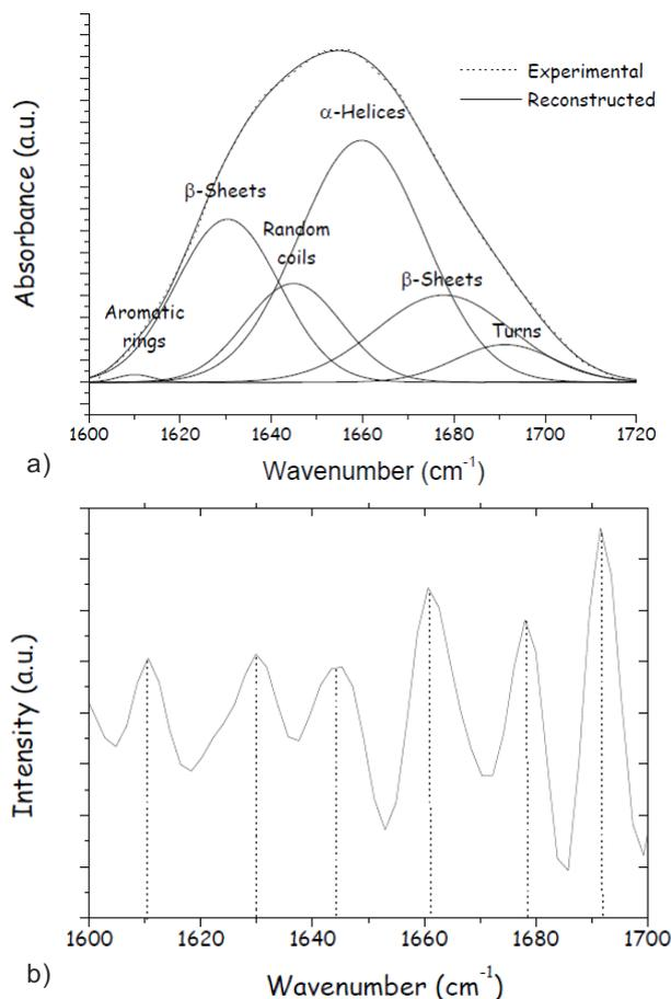
Figure 3: a) Curve-fitting analysis of the amide I profile on MBB in ATR-FTIR and b) fourth derivative function. Identification of the six components (aromatic rings,  $\beta$ -sheets (two components), random coils,  $\alpha$ -helix and turns).
