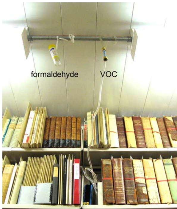
Figure 2: Formaldehyde and VOC samplers hung from light fixture.
