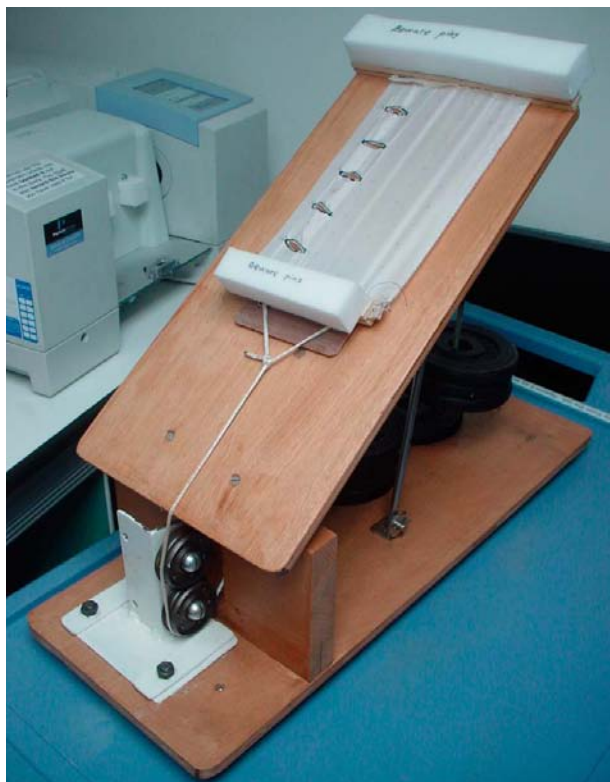
Figure 2: Typical surrogate silk object and loading rig.
