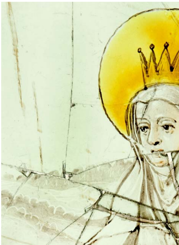
Figure 3: Detail of the reverse of the roundel showing repairs: Raman investigation characterised the unknown polymer (Figure 6) used for edge-to-edge bonding to the left of the head of St. Elizabeth.
