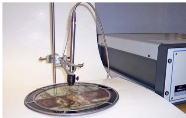
Figure 2: Analysis of epoxy resin adhesive in the roundel by means of the Perkin Elmer RamanFlex 400F instrument with a fibre-optic probe.
