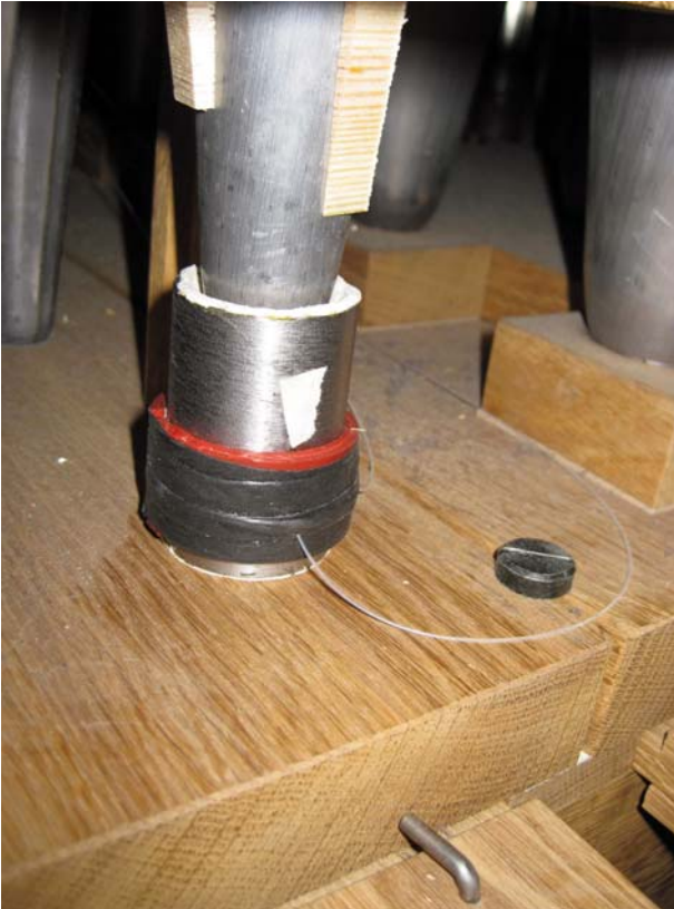
Figure 12: During the experiment, an adapter was inserted between the pipe foot and the toeboard hole in order to make easier the passage of the optical fibres and avoid any damage when handling the fibre or the pipe.
