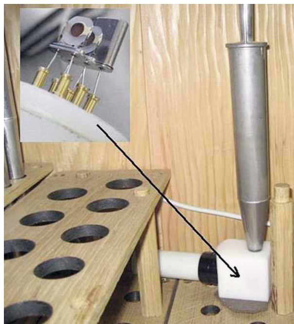
Figure 6a: View of crystal holder located at toe of pipe raised from the toeboard in the organ in St. Botolph. Top left gives view of crystals in holder.
