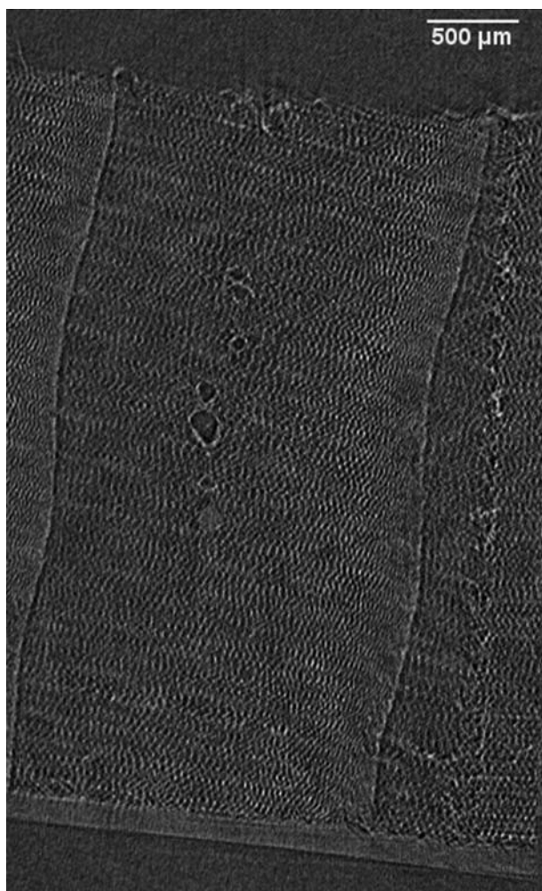
Figure 7: Slice from a Local Area Microtomography, showing a portion of the front plate between the f-holes. High resolution detail taken from the analysis of a whole violin can be appreciated, from the cellular structure and some defects of the wood to the quality of the varnish layer.
