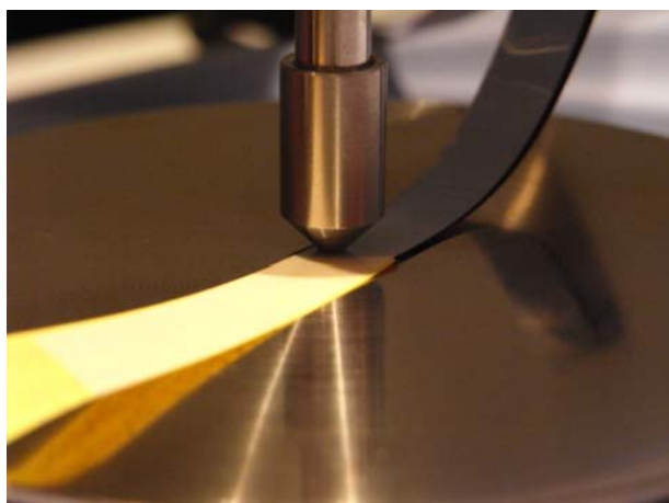
Figure 3: Acquisition of the FTIR spectrum of a magnetic tape (information side below).
