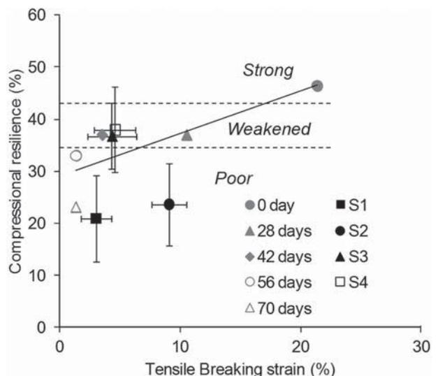
Figure 10: Relationship between tensile breaking strain and compression resilience for historic Suga-yarns (S1, S2, S3 and S4). The data points represent the averages and error bars show the standard deviations.
