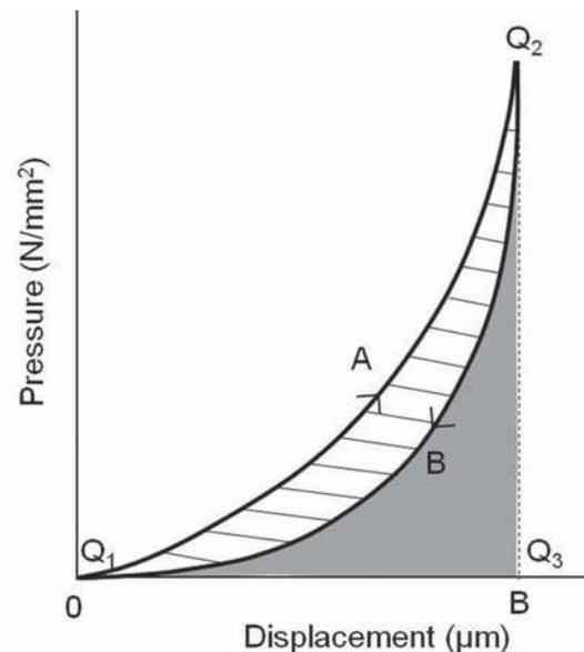
Figure 4: Typical pressure-displacement curves for the compression test. Curve A represents the compression process and B the recovery process after reaching a maximum force at  $Q_2$ . WC(Compression energy)=[area  $Q_1 A Q_2 Q_3$ ]. RC=(Compression resilience)=[area  $Q_1 B Q_2 Q_3$ ]/WC.  $\delta D$ =(Compression displacement)= $Q_1 Q_3$ , displacement at the maximum force.
