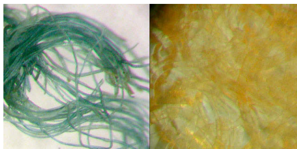
Figure 4: Photomicrographic images obtained through a stereo microscope of the turquoise yarn, as labeled in Figure 3, before dye extraction (left) and after (right).
