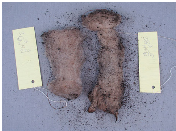
Figure 11: Sheep farm wool, mordant solution E (left, alum only) and D (right), K_2CO_3 used to extract the alkanet.
