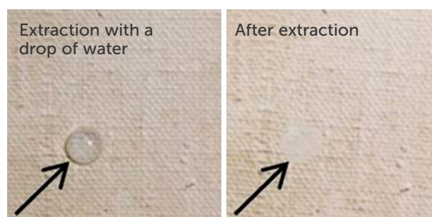
Figure 2. Aqueous extraction, locally removing the brown stains.
