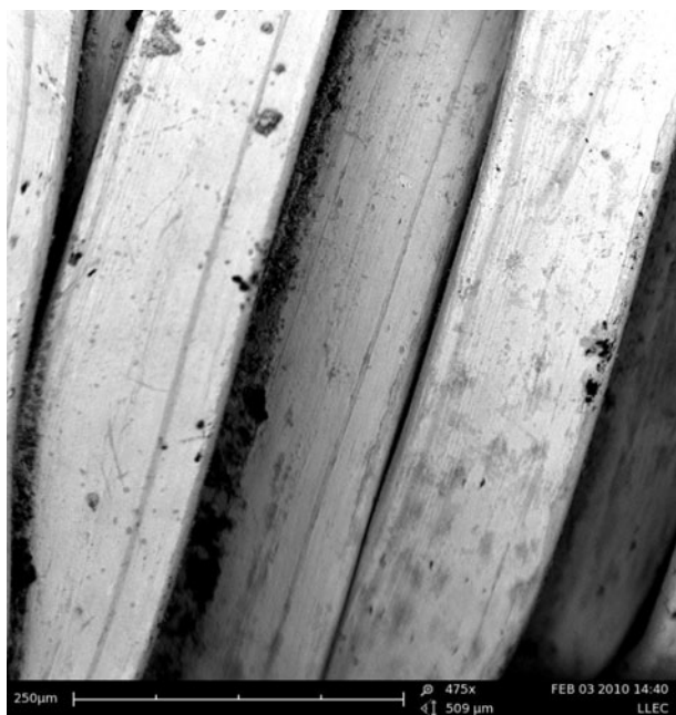
Figure 11: Show melting of the metal threads using irradiated at fluence of 2.5 \text{ Jcm}^{-2} with 12 scans.
