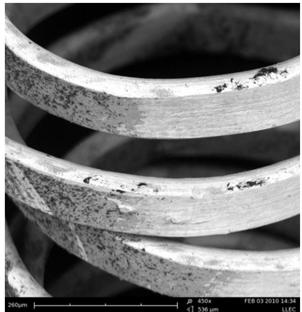
Figure 8: SEM imaging of satisfactory laser cleaning of tarnish from flattened surface of the metal threads at fluences of 1.91.
