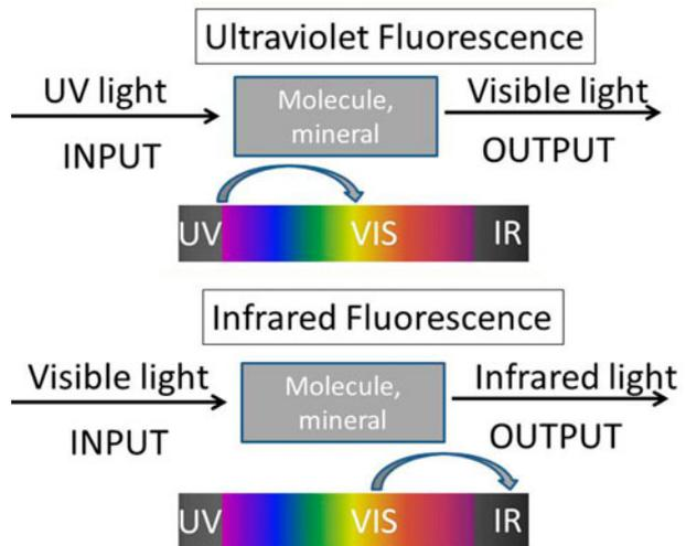
Figure 15: Ultraviolet and Infrared Fluorescence can both be described as a phenomenon where a specific light is input and another longer wavelength light is output.
