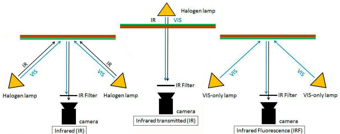
Figure 4: Equipment set up for each infrared photographic method.
