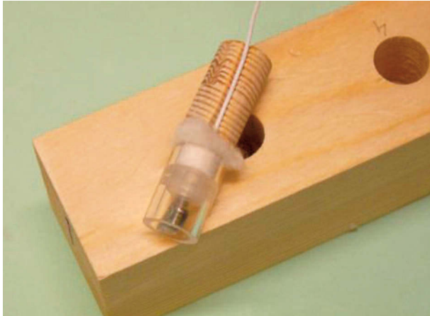
Figure 4: The small RH and T sensor can be seen in the bottom of the acrylic tube. Behind it are two silicon stopper discs, cotton wool and finally the wood plug. The setup was thereafter placed in the drilled hole of the wooden sample.
