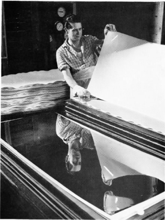
Figure 8. Polishing of celluloid sheets, from Yarsley, Flavell and Perkins, 1964, Cellulosic plastics, Plate 12. Original source: B. X. Plastics Ltd. © The Institute of Materials, Minerals and Mining (IOM3).
