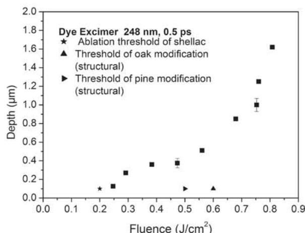
Figure 4: Ablation rate of shellac when irradiated with Dye Excimer 248 nm, (pulse duration 0.5 ps). Every datum point is an average of at least 3 to 4 different measurements. The error bars are indicative.
