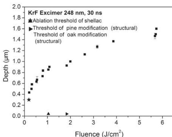
Figure 3: Ablation rate of shellac when irradiated with KrF Excimer 248 nm, (pulse duration 30 ns). Every datum point is an average of at least 3 to 4 different measurements. The error bars are indicative.
