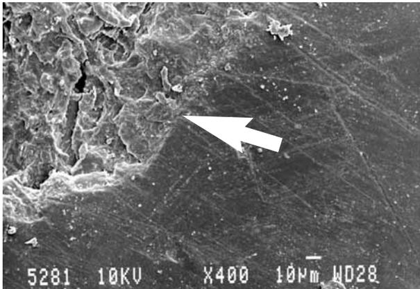
Figure 5: SEM micrograph of spot created (arrowed) on oak coated with shellac with 1 pulse. Fluence: 0.2 J/cm<sup>2</sup>. Laser: Nd:YAG 1064 nm, 1 ns. Bar = 10 µm.
