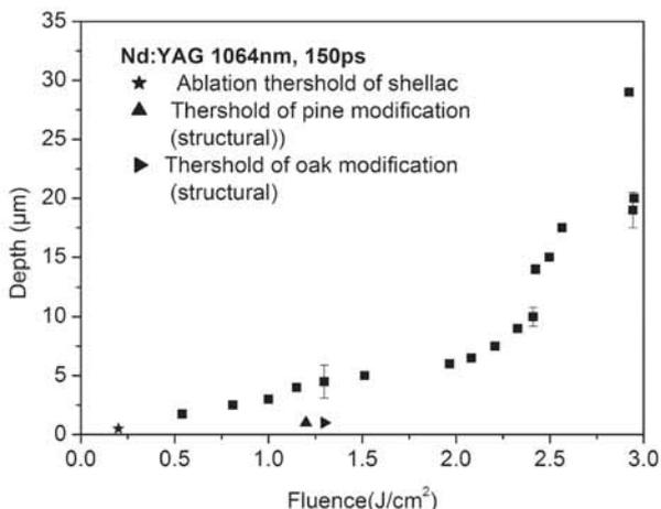
Figure 1: Ablation rate of shellac when irradiated with Nd: YAG 1064 nm, (pulse duration 10 ns). Every datum point is an average of at least 3 to 4 different measurements. The error bars are indicative.
