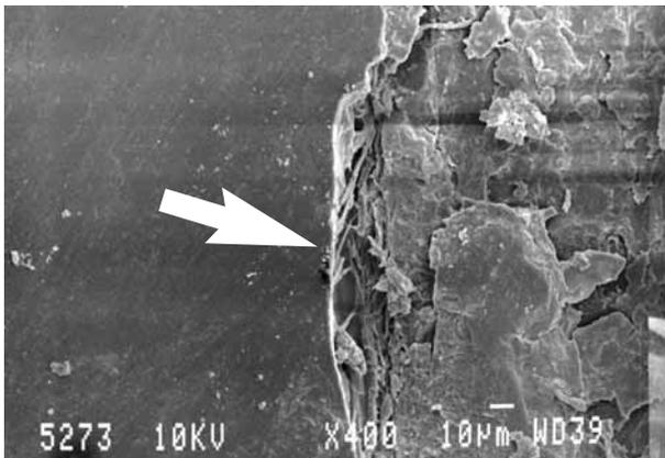
Figure 6: SEM micrograph of spot created (arrowed) on oak coated with shellac with 1 pulse. Fluence: 0.2 J/cm<sup>2</sup>. Laser: Nd:YAG 1064 nm, 150 ps. Bar = 10 µm.
