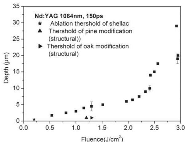
Figure 2: Ablation rate of shellac when irradiated with Nd: YAG 1064 nm, (pulse duration 150 ps). Every datum point is an average of at least 3 to 4 different measurements. The error bars are indicative.
