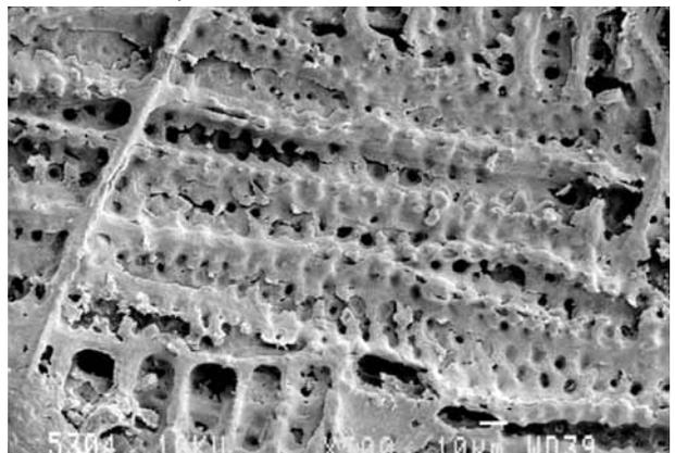
Figure 8: SEM micrograph of spot created on uncoated oak mock-up with 1 pulse. Fluence: 0.5 J/cm<sup>2</sup>. Laser: Excimer 248 nm, 0.5 ps. Bar = 10 µm.
