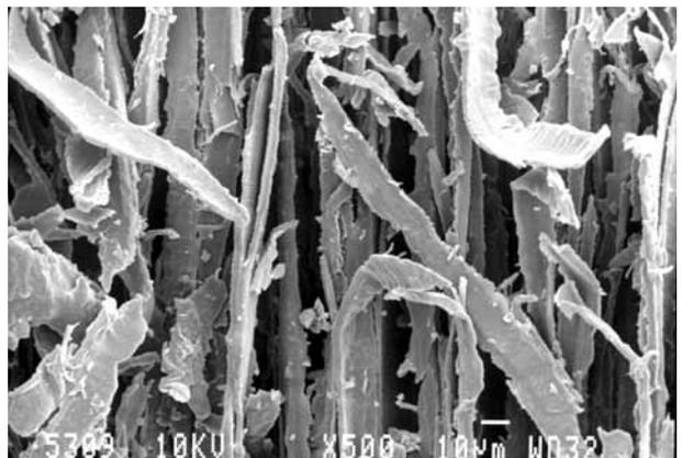
Figure 7: SEM micrograph of spot created on uncoated pine mock-up with 1 pulse. Fluence: 1 J/cm<sup>2</sup>. Laser: Excimer 248 nm, 30 ns. Bar = 10 µm.
